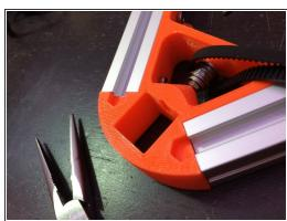
Fit the M3x25 screw through the one of the brackets and progressively add in this sequence: washer (shiny side towards bearing), first bearing (flange right), second bearing (flange left), belt, second washer (shiny side towards bearing), third washer (shiny side towards nut) and finally the standard nut.
