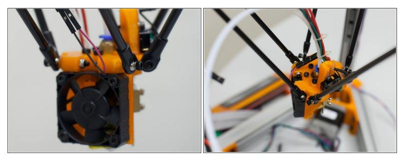
(i) Repeat several times to confirm that the probe will work reliably. You may need to grease the brass rod.
