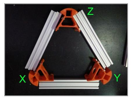
From this point on in the assembly, it is necessary to identify the 3 towers individually. Looking at the profiles with the flat LCD cables between, the front left tower will be X, the front right tower Y and the rear tower Z. The extrusions joining them will be referred to as X-Y, Y-Z and X-Z.
