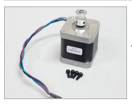
The pulley is fitted with the collar and grub screw facing towards the motor. This provides correct
