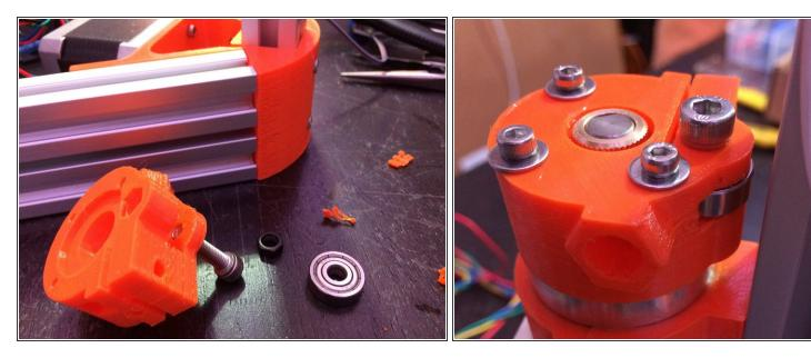
Mount the plastic extruder assembly on the stepper motor with bearing facing towards the cables, using 3 M3x25 screws.
