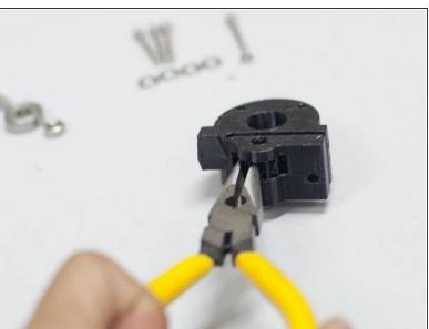
Use flat-nodes pliers, utility knife, file etc. to remove the temporary support in the extruder gap, place the 625 bearing in this slot and screw in the M5 screw/nut to hold in place. Use a sharp knife and/or a file to remove all remaining plastics until the bearing fits in tight but can run smoothly and freely.
