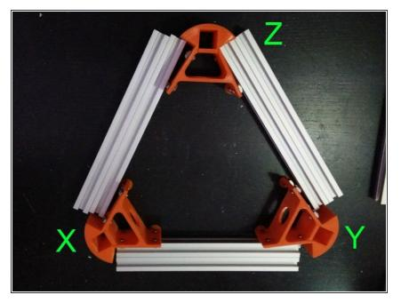
From this point on in the assembly, it is necessary to identify the 3 towers individually. Looking at the profiles with the flat LCD cables between, the front left tower will be X, the front right tower Y and the rear tower Z. The extrusions joining them will be referred to as X-Y, Y-Z and X-Z.
