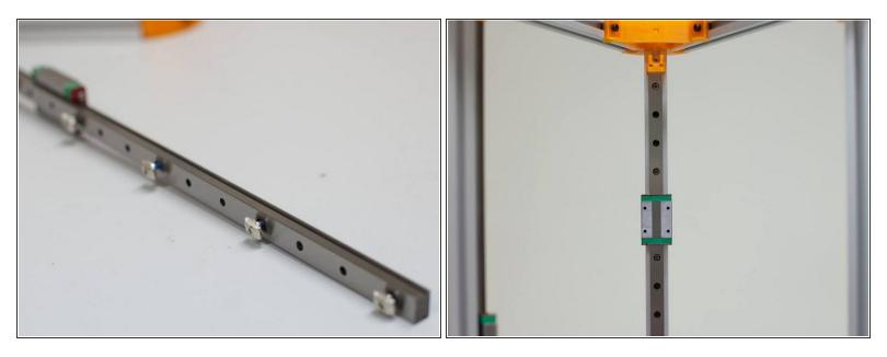
Attention: Make sure the slides don't accidentally come off the side rails when pulling them out of their covers! If it happens, it is almost impossible to re-insert the tiny balls into the ball-bearings and we cannot exchange side rails with missing ball bearings!
