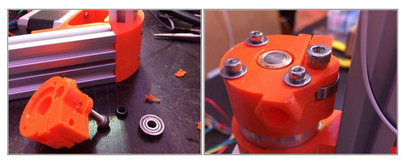
Mount the plastic extruder assembly on the stepper motor with bearing facing towards the cables, using 3 M3x25 screws.
