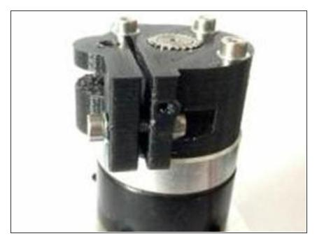
• Then horizontally mount the M3x20 screw and washer through this hole and place a nyloc nut on the end.
