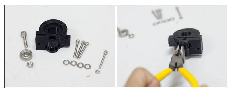
Use flat-nodes pliers, utility knife, file etc. to remove the temporary support in the extruder gap, place the 625 bearing in this slot and screw in the M5 screw/nut to hold in place. Use a sharp knife and/or a file to remove all remaining plastics until the bearing fits in tight but can run smoothly and freely.
