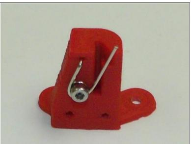
Cut off top ends of safety pin. Insert the left leg into the small hole at the top of the printed Z-probe holder and bend the pin so that the loop aligns with the hole. Secure with one of the M2.5x12 screws.
